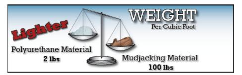
Mudjacking uses a grout based material infused with mud and Portland cement. It is hydraulically pumped under the concrete to fill in voids and raise the concrete. Foam jacking uses a polyurethane foam material that
